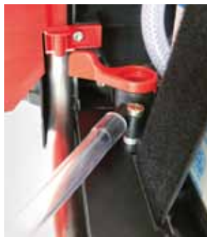
Drain hose and valve
