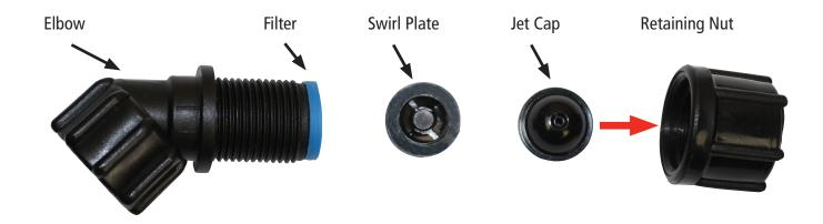
Step 3: Drop the swirl plate, on top of the jet cap, into the retaining nut
