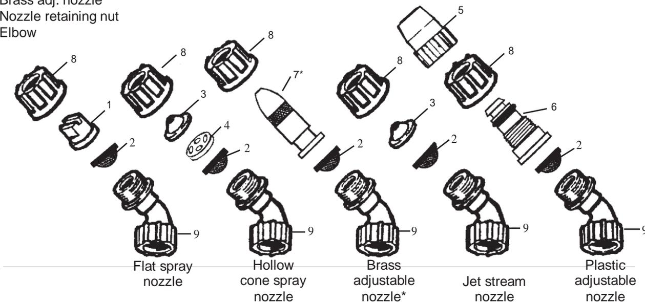
\*Brass adjustable nozzle and Speed Tip nozzle are not standard items on all Solo sprayers but each may be purchased as an accessory. Spray tips should be assembled as above for desired spray pattern.
