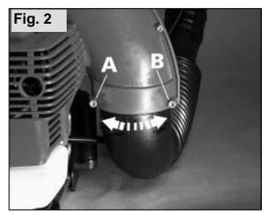
Remove screws A and B.
