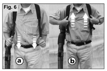
Put blower on back and secure carrying straps with quick-coupling locks (13).
