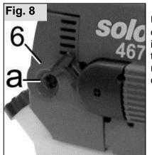
Undo the screw (a) completely (screw is retained inside the filter cover) and remove the filter cover (6).
