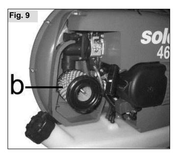
The best way to clean the filter is to simply tap out any dirt or blow it carefully out with a low blast of air.
