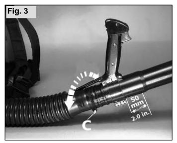
Push multi-function handle onto blower tube and fix with 2 screws in the required, comfortable position. The adjustment scope is approx. 50mm depending on the arm length of the operator.
