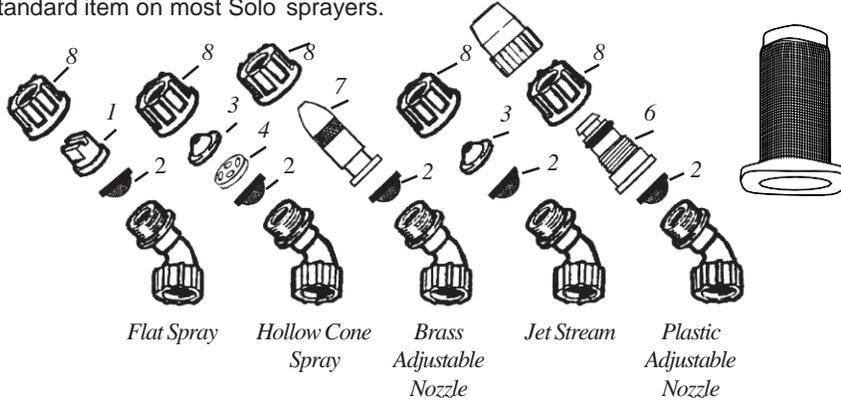
No-drip-check valve replaces # 2 on heavy-duty (HD) models along with O-rings 0062106 and 0062115.
